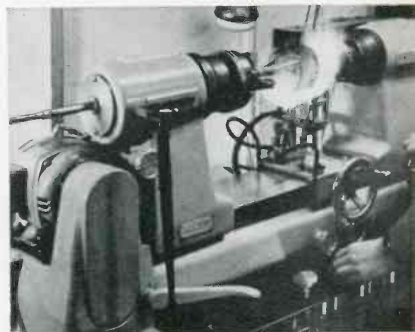
Glass bulbs are annealed after tube is fully assembled. This action relieves stress and strain in the glass itself which may be induced during manufacture.
