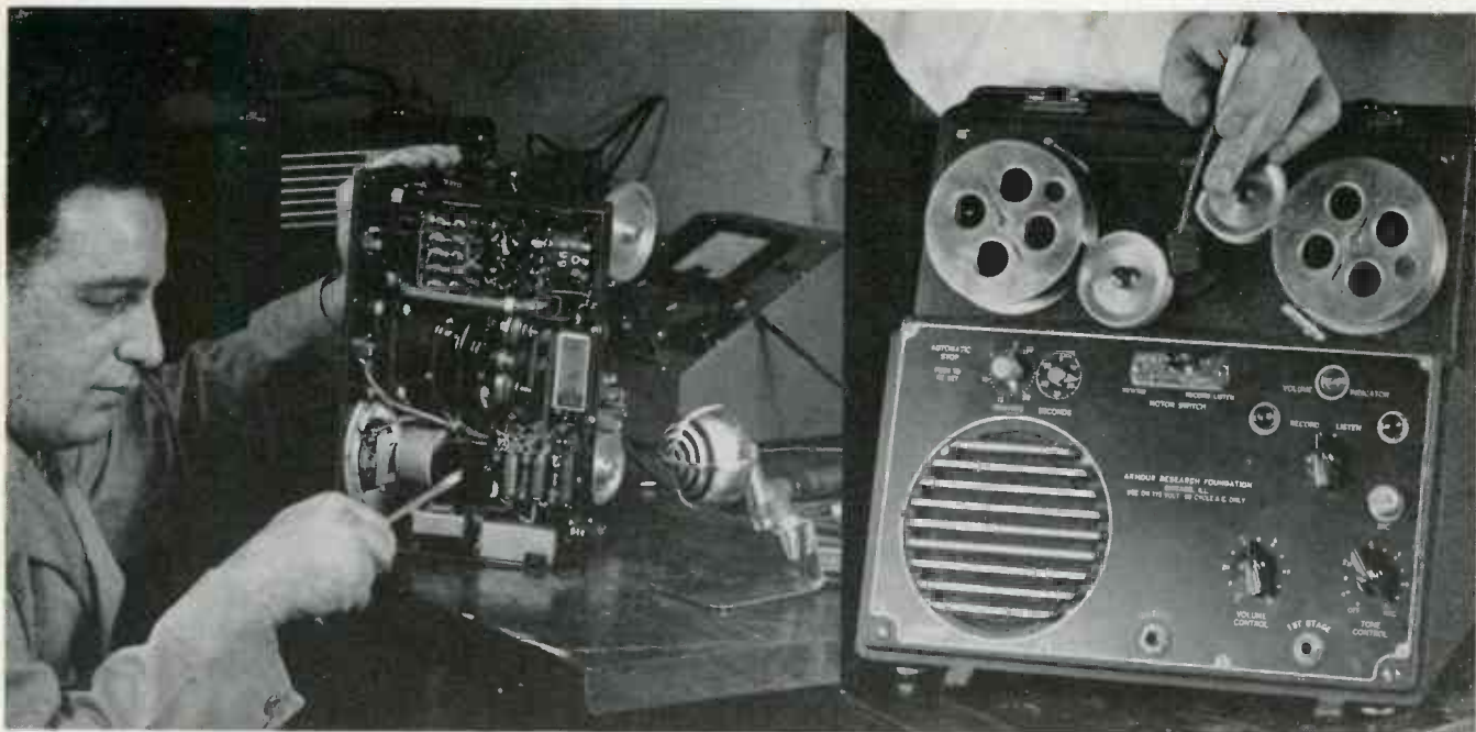
Marvin Camras of Armour Research Foundation, Chicago, and his invention, the iron-wire recorder, back and front of which are shown. Recorder differs from earlier types in its new form of recording head, indicated by the pencil
