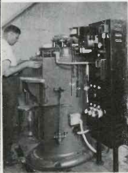
Wholly or semi-automatic waxing machine showing pilot lights and instrument control of wax and air temperatures and electrical and mechanical operations.
