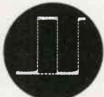
Oscillogram of the response of a given amplifier to a 100 kilocycle square-wave signal. Such electronic writing provides the best evidence of actual performance.
