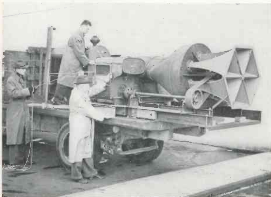
This loudest noise-machine ever built, designed by Bell Laboratories and built by Chrysler, has been on tour visiting 40 cities. It delivers alarm warnings over areas from 10 to 130 square miles. New York, Detroit, Chicago and San Francisco have installed similar noise machines as basis of their air-raid alarms. Our sound-level chart supplement, accompanying this issue, shows output of this Chrysler-Bell Victory siren to be: Close-up, 172 db; at 100 ft., 136 db (threshold of pain, 130 db); at one mile, 100 db!
