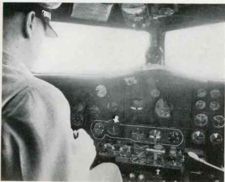
← The cross-pointer indicator as installed in the plane instrument board is shown below arrow, together with associated plane instruments
