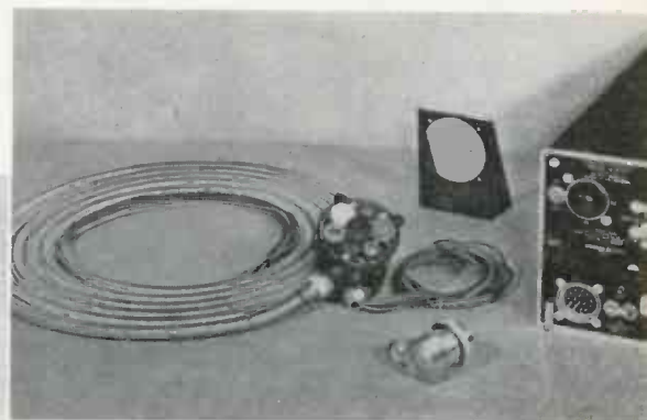
↑ Marker-beacon receiver for mounting in instrument panel of airplane equipped for instrument landing
