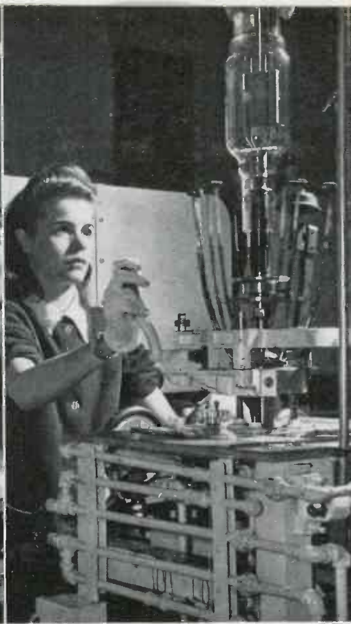
▲ TUBE-SEALING speed was doubled by switch from horizontal lathe to vertical outfit which holds tube stationary while torch cluster revolves, at Westinghouse Lamp Division
