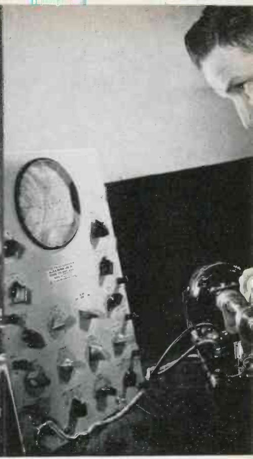
▲ FLAWS in heat-treated steel parts show up as non-uniform magnetism if part has been magnetized while rotating at high speed. Oscilloscope sweep is "in sync" with rotation, to locate defect
