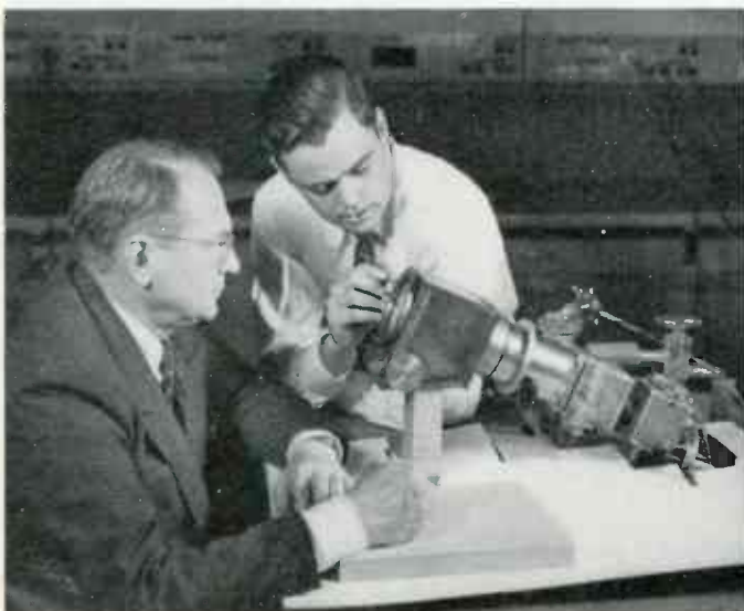
RCA's new "pocket" model, inspected by Dr. Zworykin and Dr. Hillyer. Only 16 inches long, it is capable of 100,000 magnifications, and is inexpensive enough to find wide use in smaller laboratories
